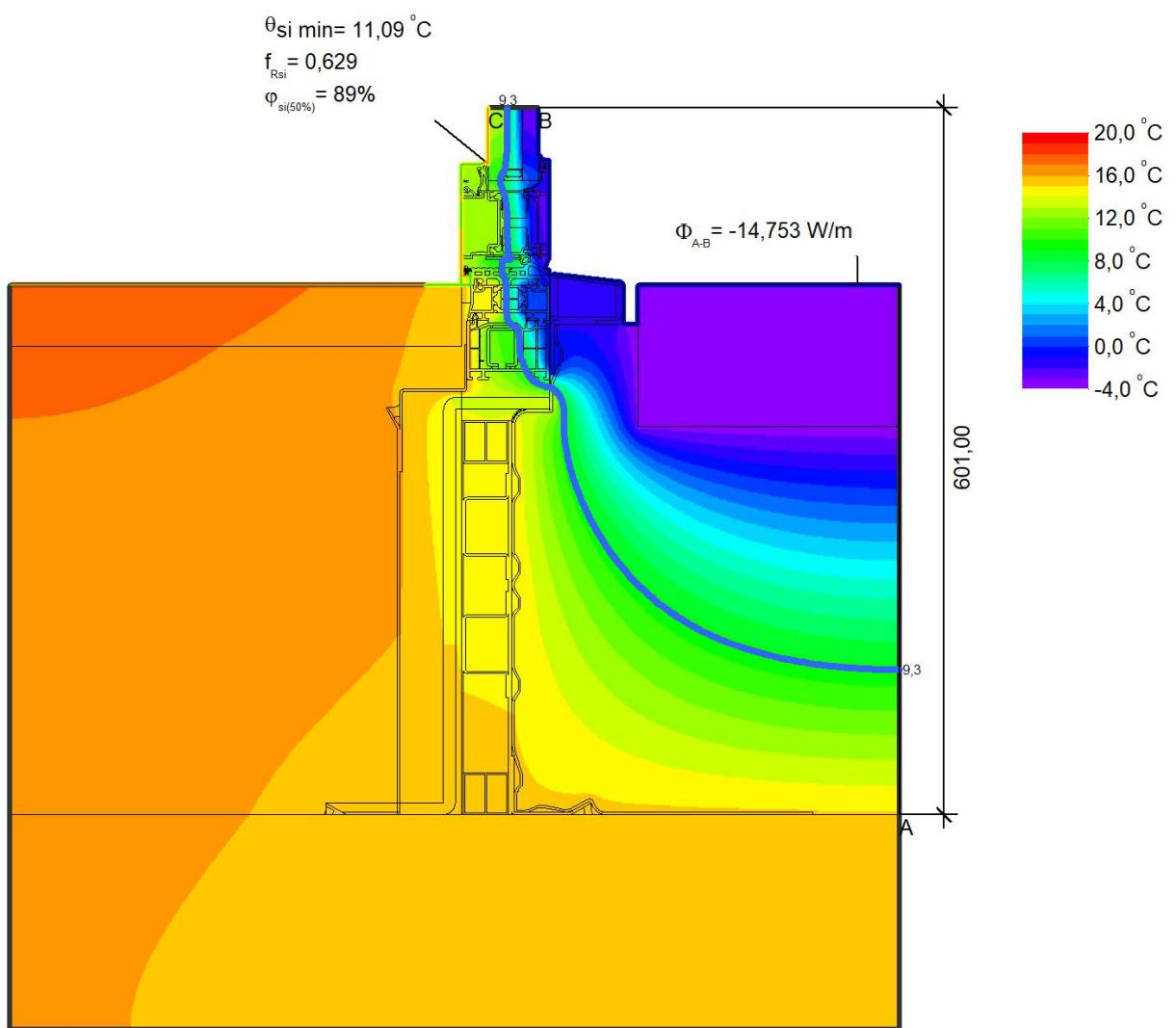
$$U_{eq \text{ A-B}} = \frac{\Phi}{\Delta T \cdot b} = \frac{14,753}{24,0 \cdot 0,601} = 1,02 \text{ W/(m}^2\text{·K)}$$
