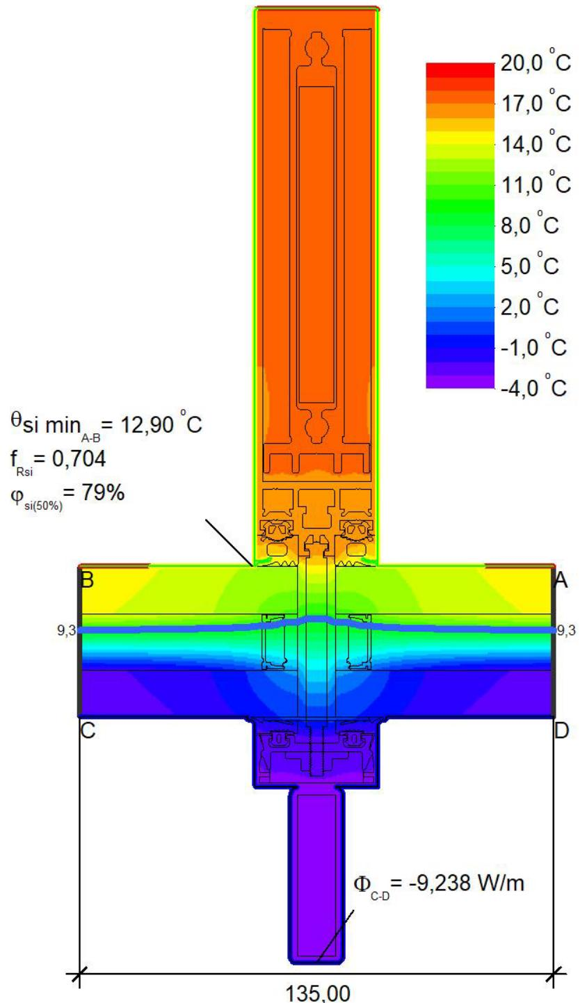
$$U_{eq \text{ C-D}} = \frac{\Phi}{\Delta T \cdot b} = \frac{9,238}{24,0 \cdot 0,135} = 2,85 \text{ W/(m}^2 \cdot \text{K)}$$
