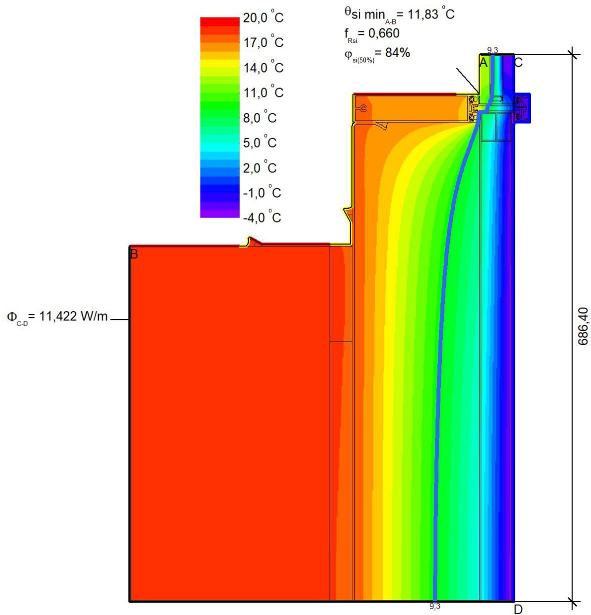
$$U_{\text{eq C-D}} = \frac{\Phi}{\Delta T \cdot b} = \frac{11,422}{24,0 \cdot 0,686} = 0,693 \text{ W/(m}^2 \cdot \text{K)}$$
