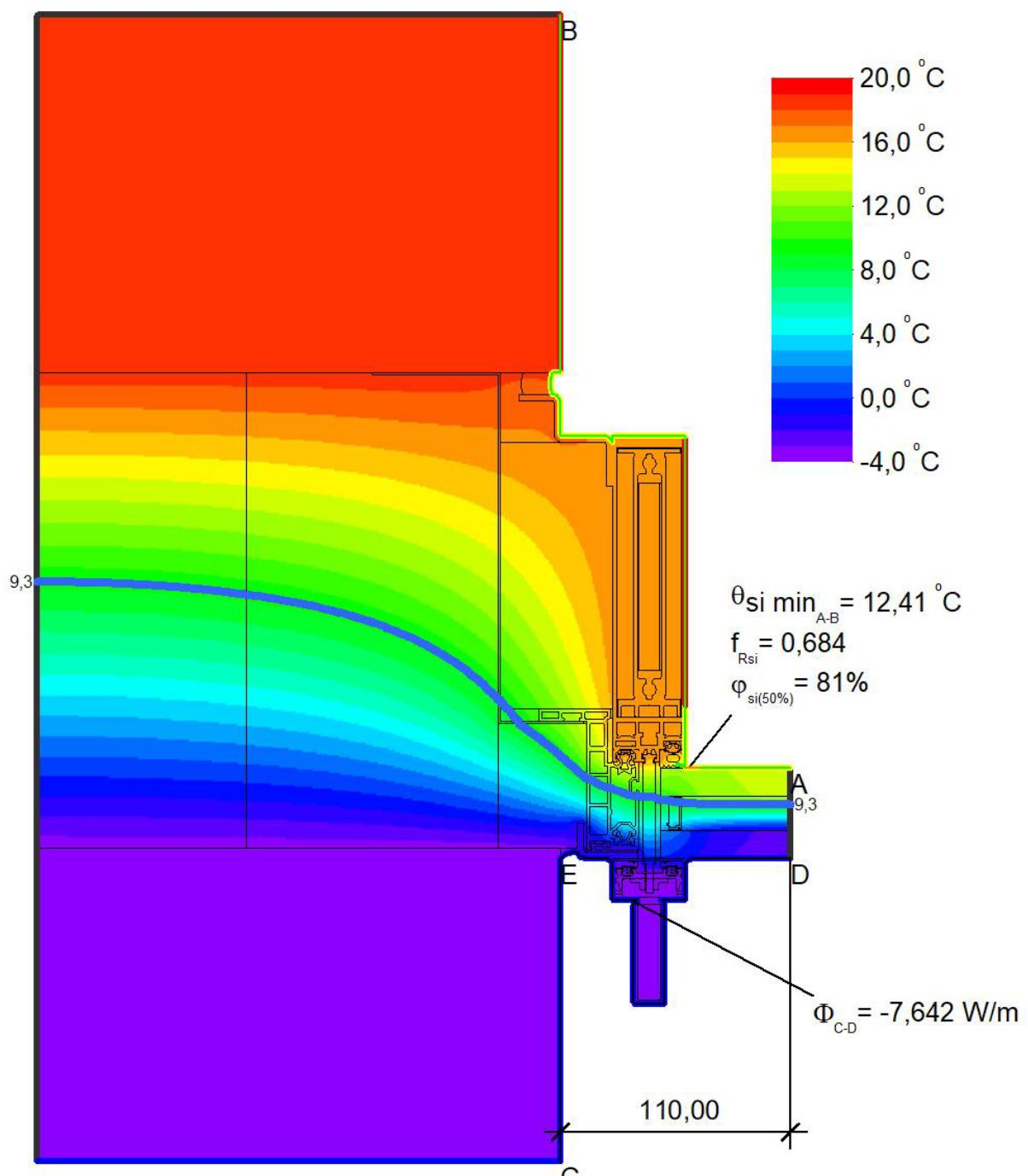
$$U_{eq \text{ C-D}} = \frac{\Phi}{\Delta T \cdot b} = \frac{7,642}{24,0 \cdot 0,11} = 2,89 \text{ W/(m}^2 \cdot \text{K)}$$
