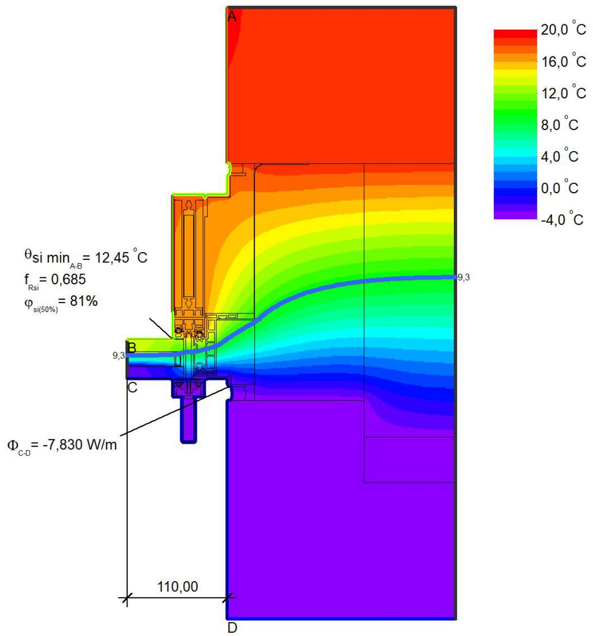
$$U_{eq \text{ C-D}} = \frac{\Phi}{\Delta T \cdot b} = \frac{7,83}{24,0 \cdot 0,11} = 2,97 \text{ W/(m}^2 \cdot \text{K)}$$
