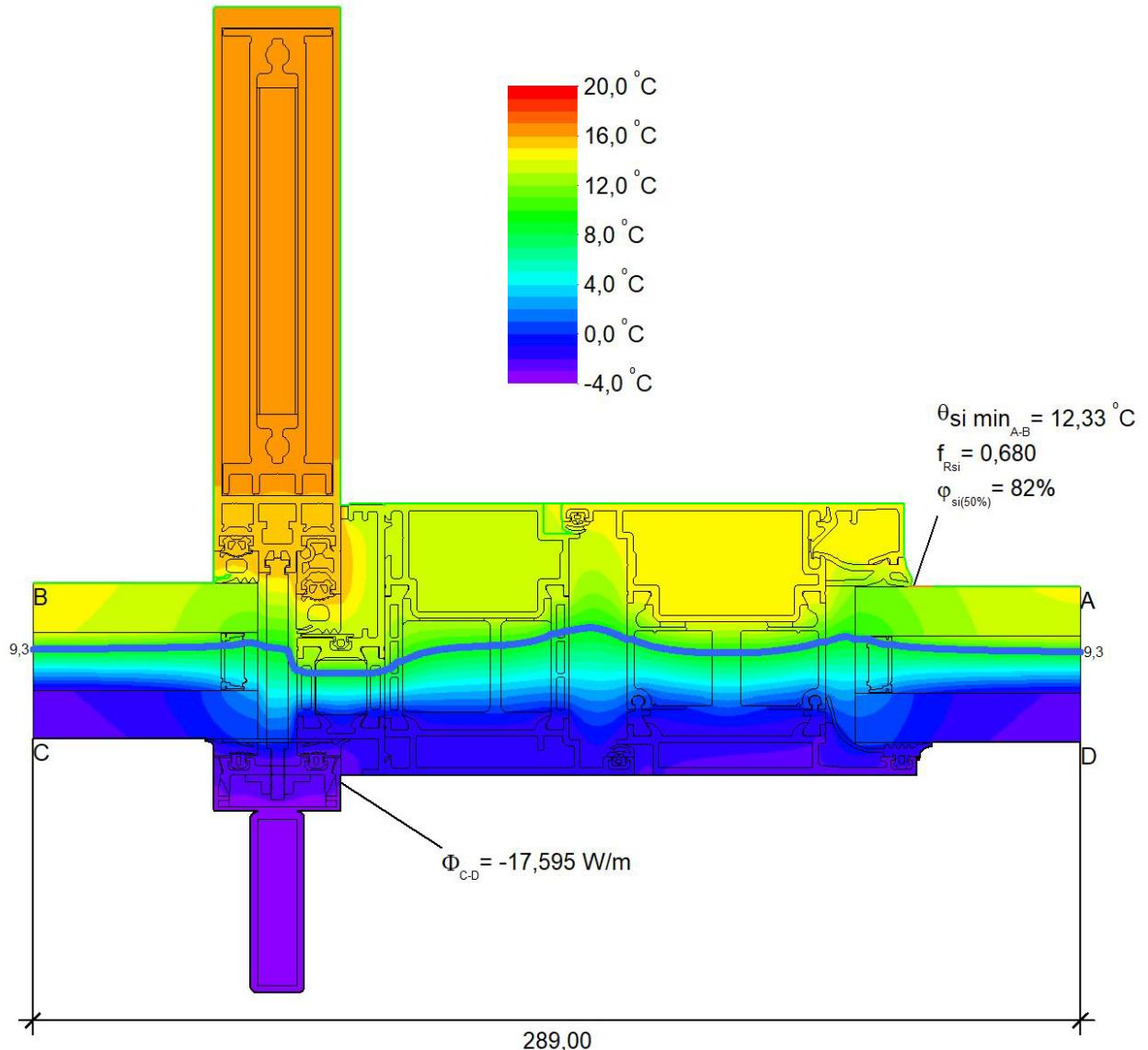
$$U_{eq \text{ C-D}} = \frac{\Phi}{\Delta T \cdot b} = \frac{17,595}{24,0 \cdot 0,289} = 2,54 \text{ W/(m}^2 \cdot \text{K)}$$
