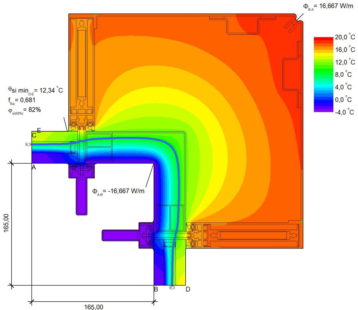
$$U_{eq A-B} = \frac{\Phi}{\Delta T \cdot b} = \frac{16,667}{24,0 \cdot 0,165} = 4,21 \text{ W}/(\text{m}^2 \cdot \text{K}) \quad U_{eq B-A} = \frac{\Phi}{\Delta T \cdot b} = \frac{16,667}{24,0 \cdot 0,165} = 4,21 \text{ W}/(\text{m}^2 \cdot \text{K})$$
