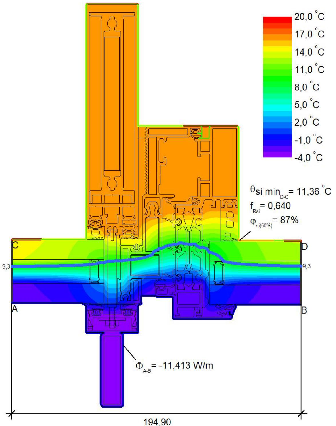
$$U_{eq \text{ A-B}} = \frac{\Phi}{\Delta T \cdot b} = \frac{11,413}{24,0 \cdot 0,195} = 2,44 \text{ W/(m}^2 \cdot \text{K)}$$
